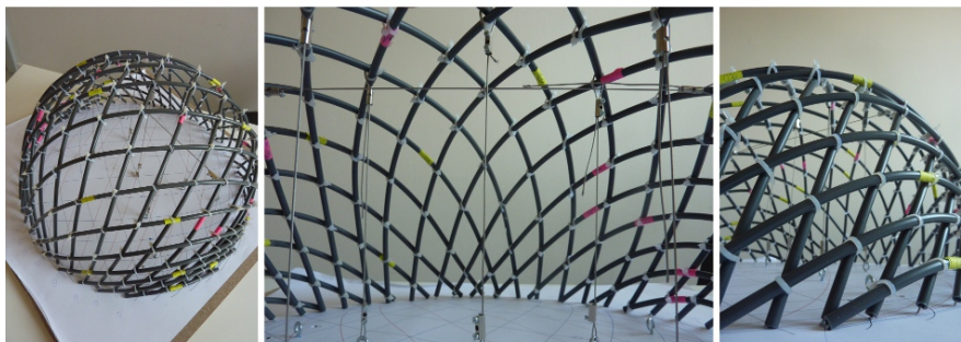
Figure 12: Physical modelling of the Flying Dome to analyse the visual effects of the irregular mesh
